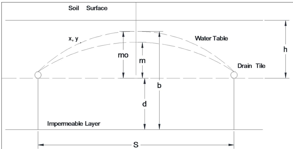
Figure 4. Cross section depiction of tile drainage system.
