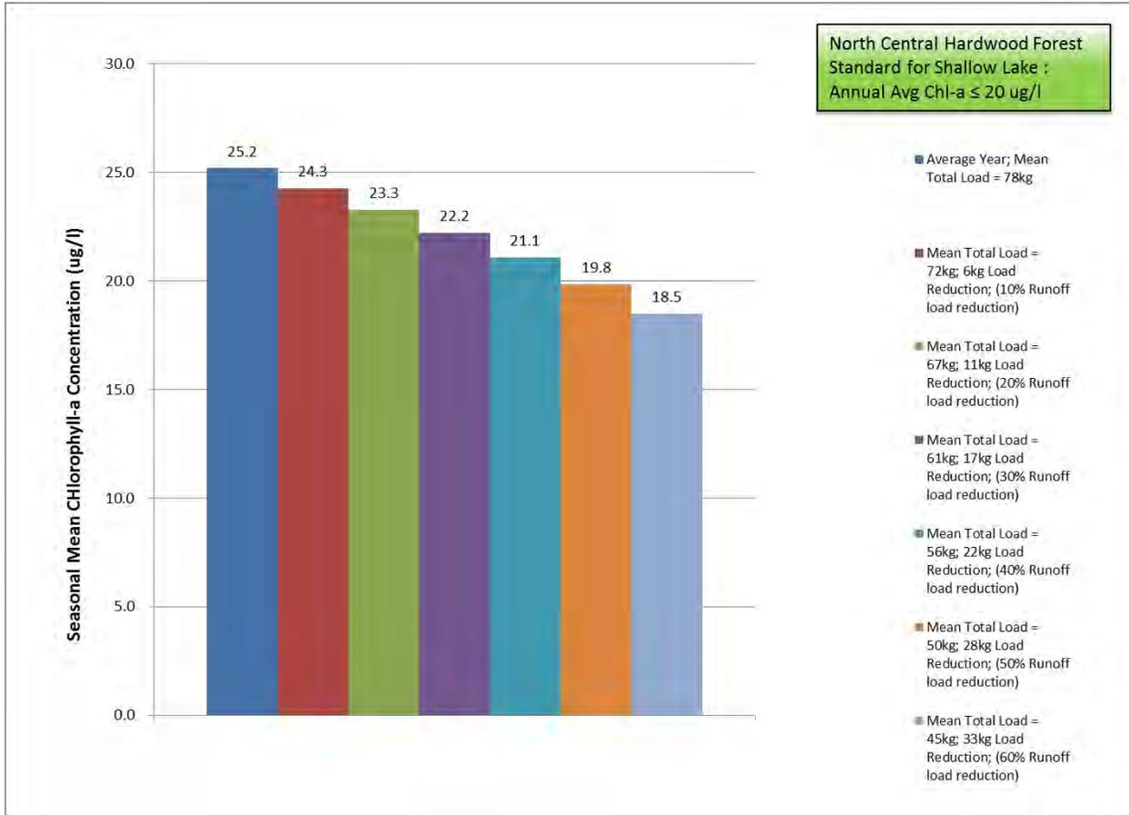
Figure 39. Adjusted Infiltration Ravine Lake frequency distribution of summer season mean chl-a concentrations under select load reduction scenarios; Simulated Conditions = 78 kg/season.
