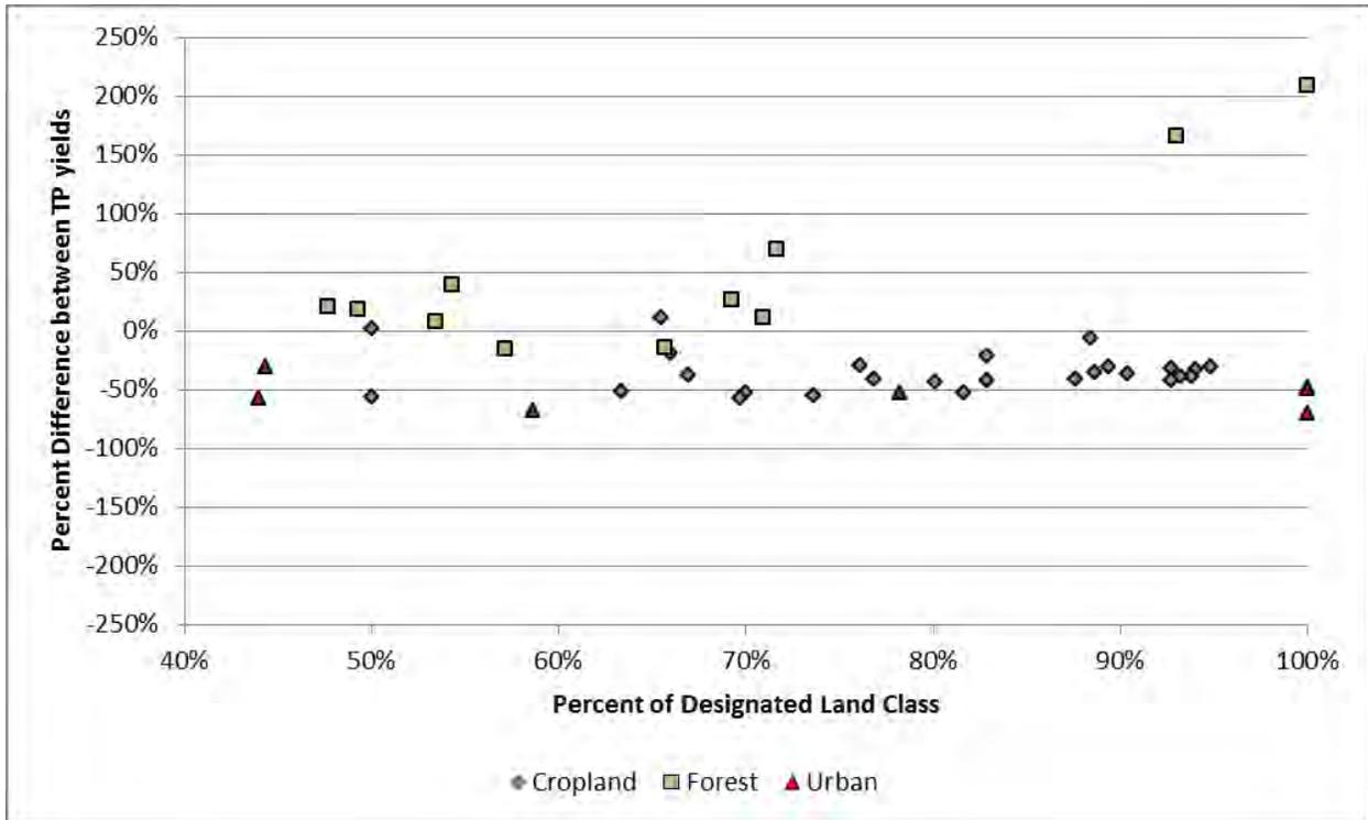
Figure 9. Future Conditions Model, comparison of simulated and expected P8 subwatershed TP yields, prior to calibration.
