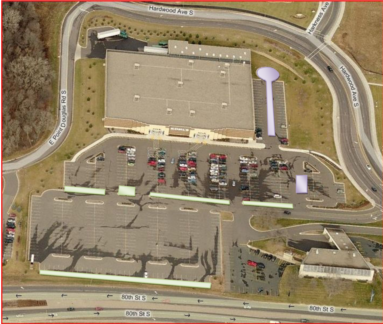
■ Proposed Bioretention Areas ■ Proposed Permeable Asphalt Areas
