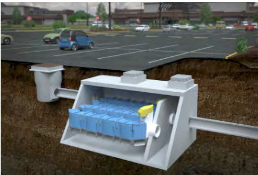
Upflo filter floats as TSS accumulates on bottom of vault. High capacity filtration media adsorb phosphorus and fine particulates. The floating rack configuration allows for retrofitting of relatively shallow pipe configurations (image Upflo).
