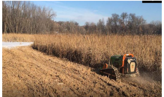
A cattail removal machine at work in a Ramsey-Washington Metro Watershed District wetland. Photo Credit: Ramsey-Washington Metro Watershed District
