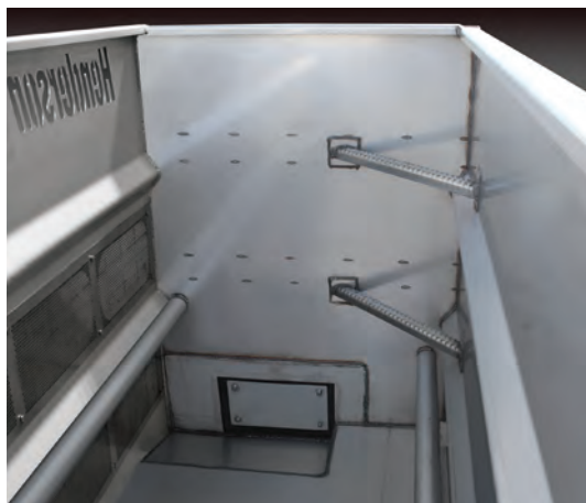
Large solids clean-out and inside ladder shown
